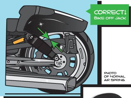
WHEN INFLATING SHOCKS FOR FIRST TIME, LOWER BIKE TO GROUND AND MAKE SURE SHOCKS ARE FULLY COMPRESSED. THEN APPLY AIR.
